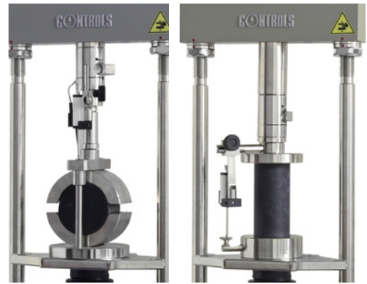
SPEEDLOADER EmS with Marshall accessories conforming to: EN 12697-34; ASTM D1559; ASTM D5581; ASTM 6927; AASHTO T245; BS 598-107; NF P98-0251-2; DIN 1996; CNR 30
