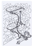
Typical application of two semi-cylindrical flat jacks with mechanical strain gauges for determining the strength and deformability features
