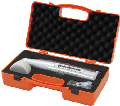
Concret test hammer ( rebard method ) 58-C0181/C
