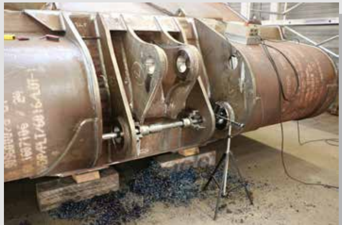
➤ Machining of the pin holes.
